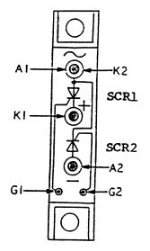
Figure 5-2. SCR Module Test Points
