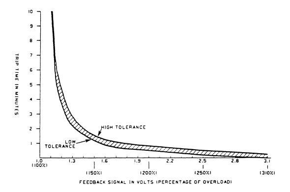
Figure 1-3. Electronic Overload Trip Curve
