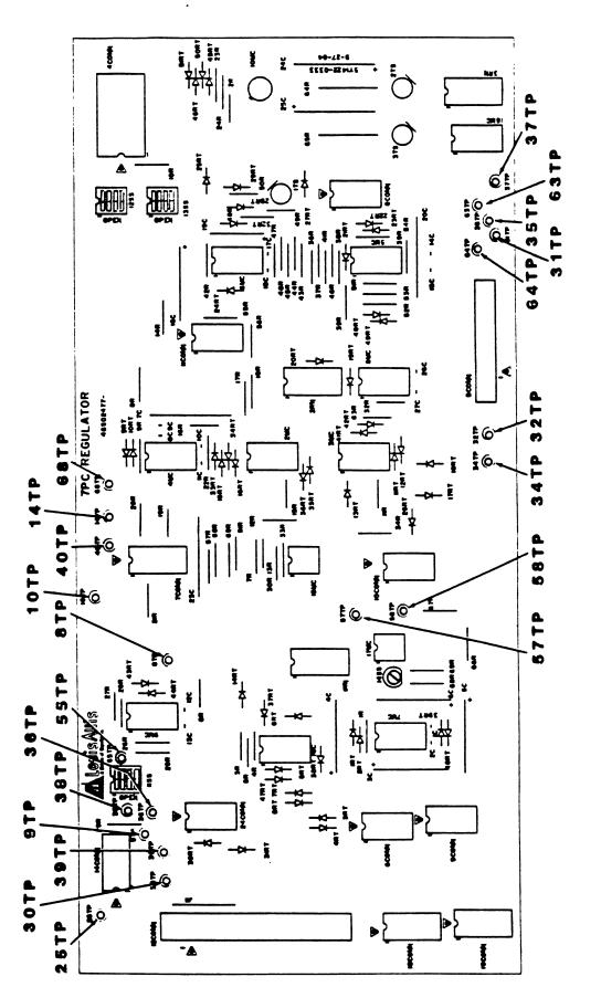
Figure 6-1. 7PC, Regulator PCB Test Point Location
