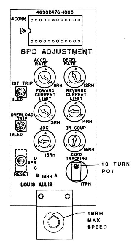
Figure 4-1. Location of Adjustment Controls
