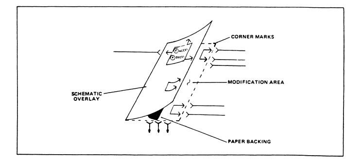
Figure 7-3. Application of Schematic Overlay
