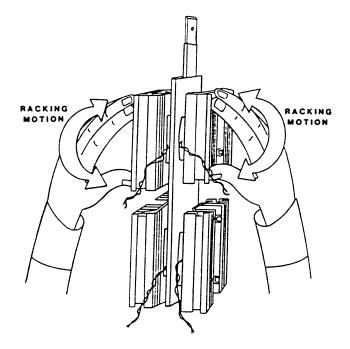
Figure 5-6. Starting Torque Check - Racking
