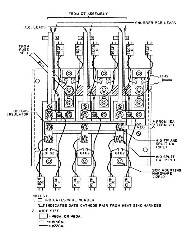
Figure 5-1. Modular Type Heat Sink Assembly and Wiring
