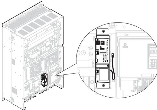
**Figure 28 Option Properly Installed**
