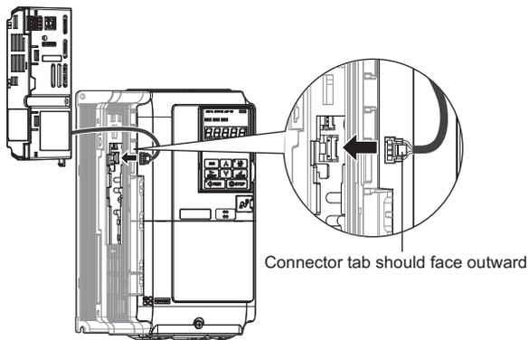
**Figure 8 Plug the Connection Cable into the Unit**
