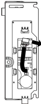
Figure 22 Pull Out the Connection Cable
