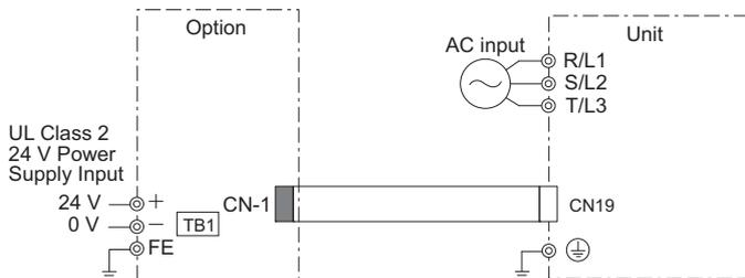
**Figure 31 Connection Diagram for Unit and Option**
