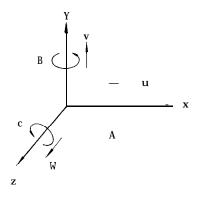
Fig. 2.1 4th Axis in Right-hand Coordinate System
