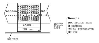
Fig. 3.4 Splicing Part Program Tape
