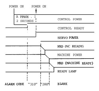
Fig. 4.11 Sequence of Turning on Operation
