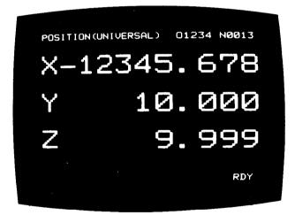
Fig. 4.19 Current Position Display (Universal) -Example
