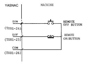
Fig. 4.13 Connections of Remote ON/OFF Pushbuttons
