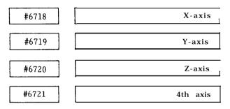
Work coordinate system setting G57 (J2) Setting : "1" = Least input increment Setting range : 0 to \*99999999
