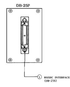
Fig. 4.39 Data 1/0 Interface Receptacles in Control Cabinet
