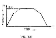
Rapid traverse rate and acceleration deceleration constant of rapid traverse rate can be set by parameter. (#6280 to #6301)
