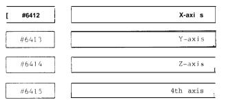
Acceleration and deceleration time constants for control unit during normal cutting are set in the order of X-, Y-, Z- and 4th-axes.
