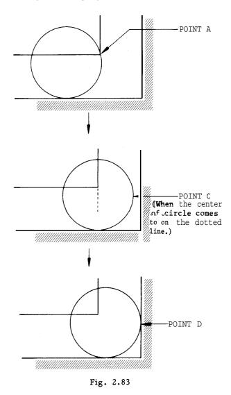
(b) When the tool radius is larger than or equal to the cutting margin
