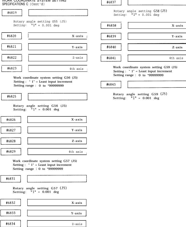
Work coordinate system setting G58 (J5) Setting : " 1" = Least input increment Setting range : 0 to ±99999999
