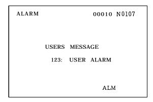
Fig. 2.78 Sample Display of Alarm Message by #8000 Command
