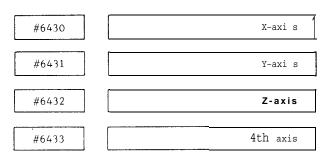
Acceleration and deceleration bias for control unit thread/tap cutting is set.
