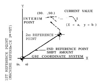
(a) First, positioning is made at the interim point (X = 30. Y= 50.). The interim point <sup>is a</sup> coordinate value of the G92 coordinate system or work coordinate system (G54 to G59).
