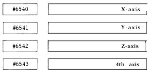
Work coordinate system setting G58 (J1) Setting : "1" = Least input increment Setting range : 0 to \*99999999
