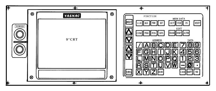
Fig. 4.1 Standard NC Operator's Panel wtth 9" CRT Character Display (Keyboard on Right Side of CRT)
