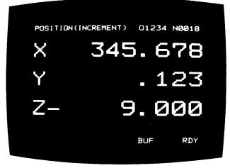
Fig. 4.21 Current Position Display (Increment) - Example
