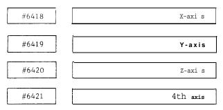
Acceleration and deceleration bias for control unit during normal cutting is set in the order of X-, Y-, Z- and 4th-axes.
