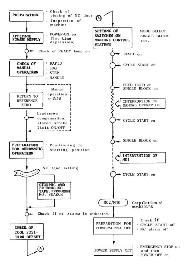
Fig. 6.5 Operating Procedure
