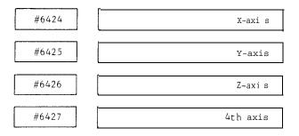
Acceleration and deceleration time constants for control unit during screw/tap cutting is set in the order of X-, Y-, Z- and 4th-axes.
