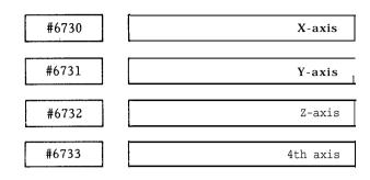
Work coordinate system setting G59 (J2) Setting : "1" = Least input increment Setting range : 0 to ±99999999
