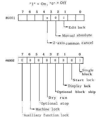
If the machine control station is provided with the switches that turn on and off the above machine functions, the state of a switch on the machine's control panel is ORed with that of the NC operator's panel will determine the machine condition.
