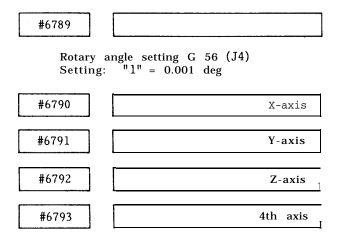
Work coordinate system setting G57 (J4) Setting : "1" = Least input increment Setting range : 0 to \*99999999
