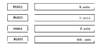
Work coordinate system setting G59 (J4) Setting : " 1" = Least input increment Setting range : 0 to \*99999999
