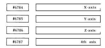
Work coordinate system setting G56 (J4) Setting : "l" = Least input increment Setting range : 0 to \*99999999
