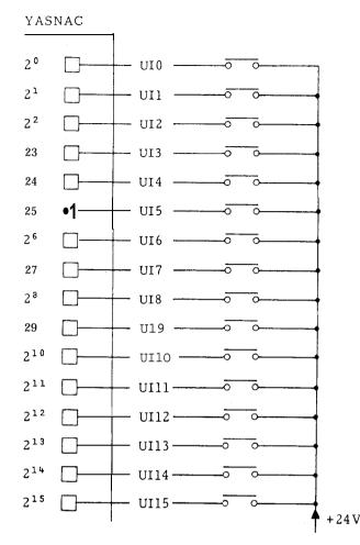
Each read variable is 1. 0 or O. 0 when the associated contact is "closed" or "open" respectively, regardless of the unit system of the machine.
