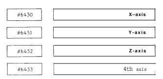
Minimum unit of travel in the order of X-, Y-, Z- and 4th-axes.
