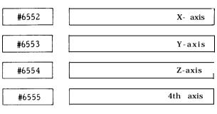
Coordinate value at skip signal ON Setting : "1" = Least input increment Setting range : 0 to \*99999999
