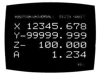
Fig. 4.20 Current Position Display ( External) -Example (with 4-axis control)
