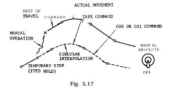
The parallel shift is reset by executing Reference Point Return manually, automatically by G28, or operating the **RESET** key. The command value is forced to change to the current position.
