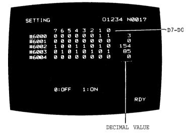
Fig. 4.24 Setting (Decimal model) -Example
