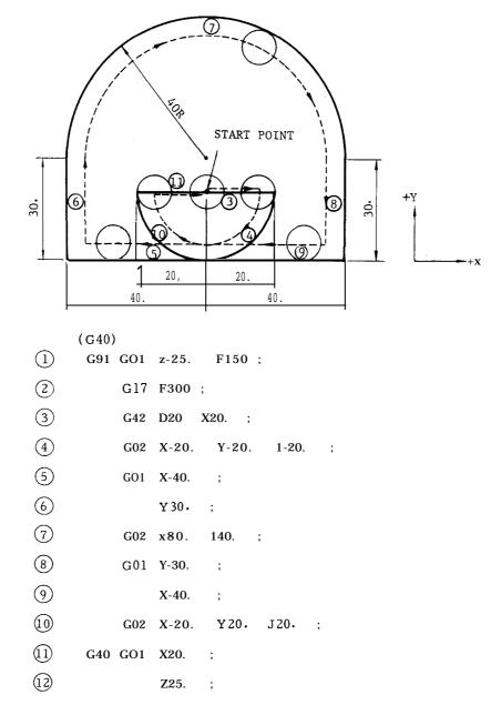
With the inner cutting in EXAMPLE A, the double cutting allowance at the cutting start and cutting end varies with the tool radius. An inner cutting case with zero double cutting allowance regardless of the cutter radius is shown in EXAMPLE B.
