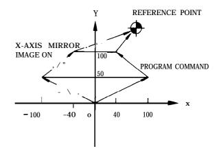
Note : When commanding axis designation under the mirror image mode (M95) by m code, stop the look-ahead by parameter (#61 16) of the set/reset M codes.
