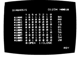
Fig. 7.4 Example of Input/Output Signal Display
