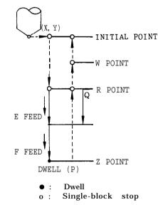
E : 2-step feedrate (1st step: E, 2nd step: F) Speed switching point (incremental) Q : w :
