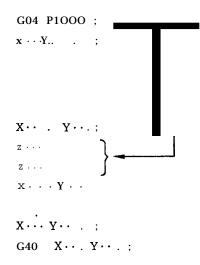
Blocks without movement in compensation plane. (When these blocks are within two, machining is made smoothly.)
