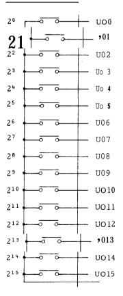
When 1.0 or 0.0 are substituted in any of #1100 through #1115, the associated output contact is output in the "closed" or "open"state.
