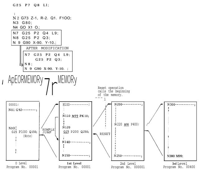
Note: Always use the program number in the P command when commanding from a tape. Example: N1OG25 P<u>01</u>0100Q1550; Program,number
