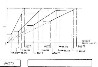
Specifies the spindle motor speed in effect when a spindle orientation (SOR) input is entered (specifiable in S5-digit designation).
