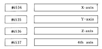
Work coordinate system setting G57 (J1) Setting : "1" = Least input increment Setting range : 0 to \*99999999
