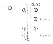
Linear form acceleration /deceleration is automatically applied to the spindle movement (the constant set by #6291).
