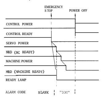
Fig. 4.12 Sequence of Turning off Operation
