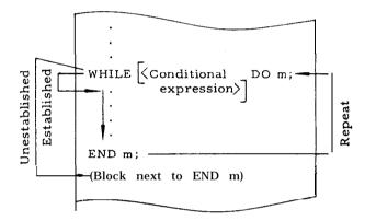
When the specification is made omitting WHILE [< conditional expression>], the blocks between DO m and END m are repeated infinitely. Generally, this is used in the format shown below .
