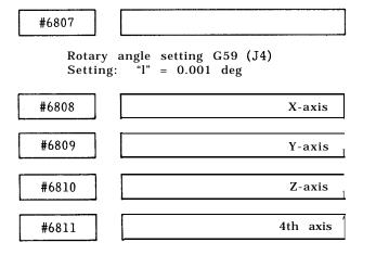
Work coordinate system setting G54 (J5) Setting : "1" = Least input increment Setting range : 0 to ±99999999
