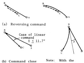
Command close to reversing circular arc command, tangent angle  $\theta$  alone is insuffi-
