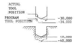
2. G45 to G48 extend and reduce the movement value programmed in the block, in the direction of movement by the tool offset value.
