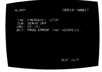
Fig. 4.29 Alarm Codes and Message Displayed-Example
