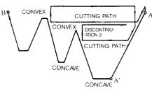
The maximum number of interrupted points that, allows cutting is three, beyond which cutting is disabled, causing "097" error. Within this limitation, any number of concaves is allowed.
