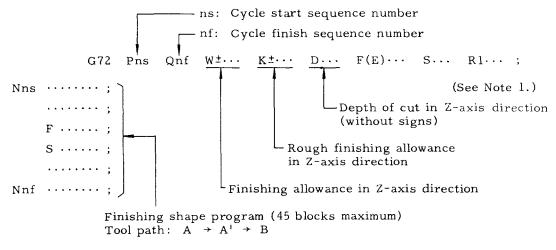
Note 1: If "R1" is specified, cutting path is computed for the concaved finishing shape program.
