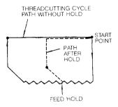
If the thread cutting hold option is not selected, depressing of the FEED HOLD during thread cutting does not hold the operation, which stops at point C where the retracting operation is completed.
