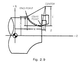
Circular interpolation of an arc on multiquadrant can be programmed in a single block.
