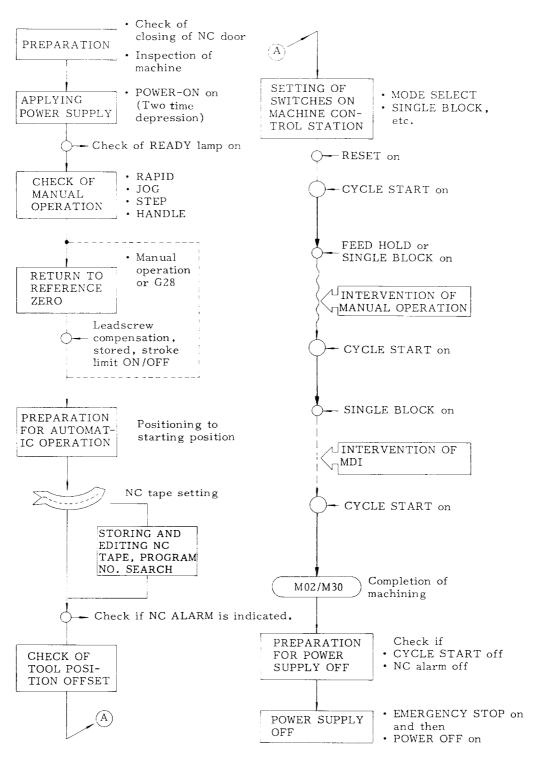
Fig. 6.1 Operating Procedure
