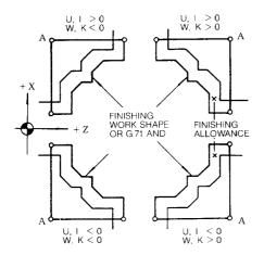
Fig. 2.47 Relation between Finishing Shape Program and Signs of Addresses U, W, I and K
