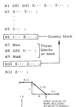
Namely, specify incremental commands I and K, which are equivalent to N10 block command, in N6 for the dummy block.
