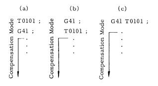
b. At the start of compensation, the tool center is offset onto the normal of the origin of the block G41 to G44 which entered the compensation mode first or of the block immediately after T code. The offset is made to the right of tool advancing direction when T+ is specified and to the left when T- is specified.
