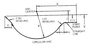
G112  $X(U) \cdots I \cdots K \cdots C \cdots D \cdots R \cdots$ ;
