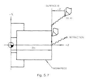
1. Push the CURRENT VALUE STORE button again, and then, retract the tool and stop the spindle.
