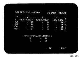
Fig. 5.10 D 2 nd screen (tool offset shift memory display screen)
