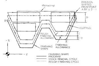
G71 starts at point A, executes the rough cutting cycle (----) and the rough finishing cycle (---), and returns to point A to be terminated. If I is not specified, the rough finishing cycle is skipped. Retracting is performed by rapid traverse G00. Thrust motion depends on the speed (G00 or G01) specified by the program of AA'. Each depth of cut D along X-axis can be overrided by 10% step within the range of 0 to 200%, by G71/G72 cut depth override selection or setting. See item (3), g.
