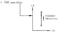
4. Values of F command at linear or circular interpolation represent the tangential feedrate when two axes are simultaneously controlled. EXAMPLE 1
