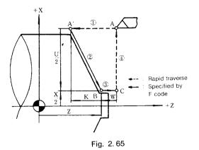
The sign of figure following the address K is decided by the direction of position A' viewed from position B.
