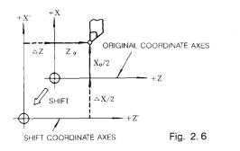
For positive shift values  $\Delta X$  and  $\Delta Z$ , the coordinate axes are shifted in the direction shown above. Xo and Zo are original coordinate system setting values.
