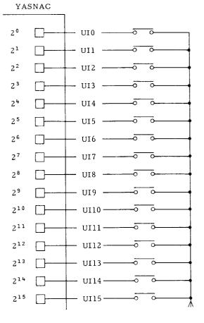
Each read variable is 1. 0 or 0.0 when the associated contact is "closed" or "open" respectively, regardless of the unit system of the machine.
