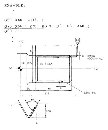
Depth of cut for each cycle when a (fixed amount) is 0.2 mm
