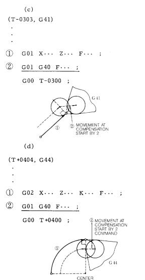
Note that, for each of above examples (a) through (b), the tool center is temporarily offset onto the normal line to the end point of the block immediately before G04 or  $T \square 00$  command.
