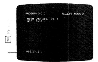
Referred to as "the data which has, just been entered" (32 characters maximum). Enter  $\overline{N}$ ,  $\overline{1}$ ,  $\overline{0}$ ,  $\overline{1}$ ,  $\overline{2}$ ,  $\overline{-}$ ,  $\overline{1}$ ,  $\overline{0}$ ,
