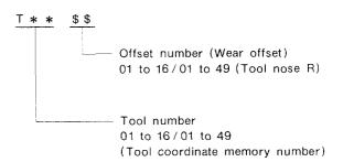
Note: The tool coordinate memory number is: (tool number + 50). Thus, the tool coordinate memory value selects the contents of (tool number + 50).
