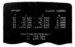
Fig. 4.32 Display of Tool Offset Amount
