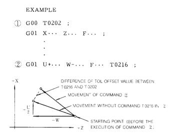
When the T command and the move command are issued in the same block, the tool nose moves to the offset position. Therefore, in the above case, the taper angle is corrected by the difference of the offset value between T0202 and T0216.
