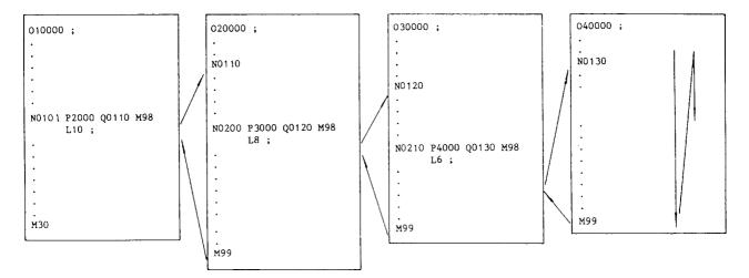
CRT screen displays that the subprogram has executed the 3rd level one time and entered into the execution of 3rd time of the 3rd level
