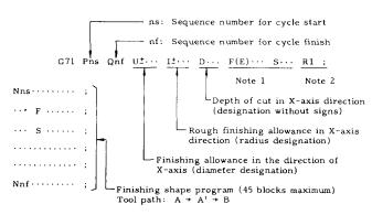
Note 1: Specifies the feed command (F(E)) and spindle command (S) for the execution of stock removal cycle.
