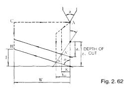
For the threading along the angle of thread, the K for each cycle obtained from the following formula should be programmed.
