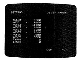
Fig. 4.36 Display of Setting Data in Decimal Mode
