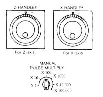
Parameter  $\#6009 D_4$  can permit setting any multiplication factor when MANUAL PULSE MULTIPLY switch is set at X100. Multiplication factor is set by parameter #6223.
