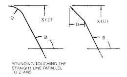
(ii) The second straight line is specified with B and Z(W).
