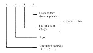
Note: The decimal point may be omitted in actual programming. For making a program including decimal points, refer to 2.1.3 Decimal Point Programming.
