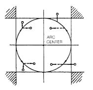
Note that if the end point is designated in the shaded area, the alarm is not displayed and the tool will continue to move endlessly.
