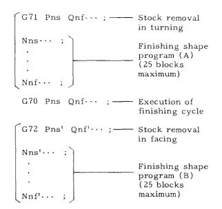
After executing the above program the program (A) is eliminated and the program (B) is retained in the finishing shape memory. Therefore, the finishing command with G70 in the trailing program is effective for the finishing shape program (B). If the sequence number specified by G70 does not match the sequence number in the memory for finishing shape program, an error ("091") is caused.
