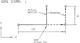
b. When the next block is programmed in absolute values only for one axis:
