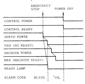
Fig. 4.13 Sequence of Turning off Operation
