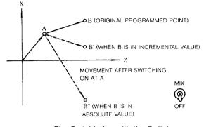
Fig. 5. 4 Motion with the Switch Turned on at Point A
