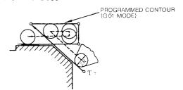
d. Command involving no movement in compensation mode
