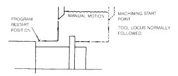
For the manual tool motion, turn on the MAN-UAL ABSOLUTE switch. If this switch is not turned on, the PROGRAM RESTART position will be shifted by the distance covered by the manual motion. For the manual motion required to avoid tool collision on the workpiece as described above, the following procedure is recommended.
