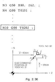
If the coordinate system setting is performed with the reference tool and tool position compensation is applied to the other tool as shown above, the tool movement may be programmed on a single coordinate system for all tool noses.
