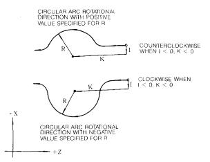
d. Address words X(U) and Z(W) are used to make discrimination between radius measuring circular arc and front circular arc. They cannot be omitted if the end point and the start point are on the same coordinates ("U0" or "W0" should be specified). When the address words other than X(U) and Z(W) are omitted, the following results are obtained:
