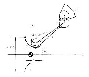
c. If the block of G41 (or G42 through G44) satisfying the compensation mode condition does not have the move command, the compensation starts and the tool center is moved on the normal.
