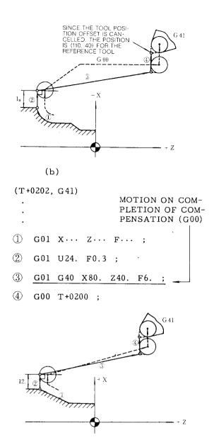
c. If the block of G40 (Nose radius compensation cancel) does not have the move command, the virtual tool nose moves to the specified end point.
