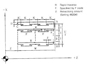
The cycle starts and finishes at position A. The fixed amount of pecking is set by the parameter No. 74.
