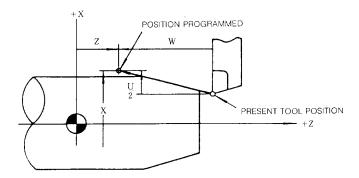
EXAMPLE G50 X100. Z60. ; G00 T0202 S600 M03 ; X35. Z5. ; G01 Z0 F1. ; Executed by linear inter-(2)X60. F0.2 ; polation G01. + X 2 5 60 DIA 35 DIA +2
