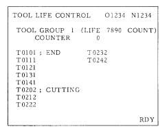
Fig. 2.72 Display of Tool Offset Memories Used for One Tool
