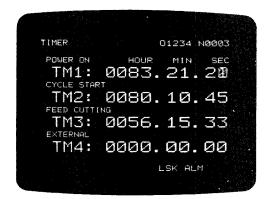
Fig. 4.43 Operation Time Display
