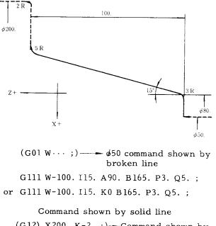
(G12) X200. K-2. ;)—Command shown by broken line after the command shown by solid line 2.8.30.2 Circular Arc Multiple Cornering (G112)
