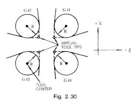
Regardless of the mode of tool nose radius compensation, the current position of the virtual tool nose is displayed by depressing the POS pushbutton.
