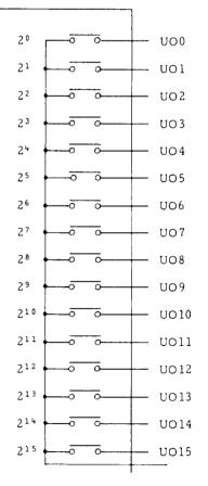
When 1.0 or 0.0 are substituted in any of #1100 through #1115, the associated output contact is output in the "closed" or "open"state.
