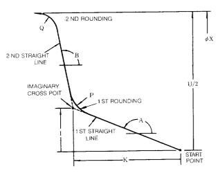
$Gill X(U) \cdots I \cdots A \cdots B \cdots P \cdots Q \cdots ; \\ Glll X(U) \cdots K \cdots A \cdots B \cdots P \cdots Q \cdots ; \\ Glll X(U) \cdots I \cdots K \cdots B \cdots P \cdots Q \cdots ;$
