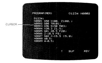
Fig. 4. 21 Display of Part Program in Memory Operation
