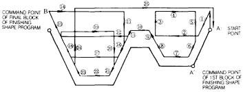
Since cutting starts with the concave nearest the start point, the cutting path is interrupted if it hits the convex beyond the concave. The concave is cut to its bottom. Then, the cutting cycle returns to the interrupted point to perform cutting beyond it.
