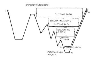
Sample Contour Not Allowing Cutting ing
