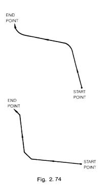
(1) Command format for configurations for multiple cornering
