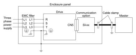
Figure 11.2 Option Installation for CE Compliance: GA500, HV600
