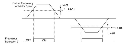
Figure i.6 Frequency Detection 2 Time Chart
