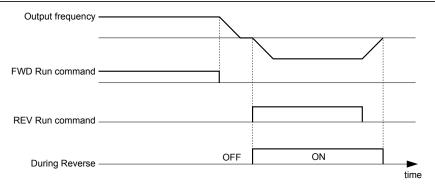
Figure i.11 Reverse Direction Output Example Time Chart
