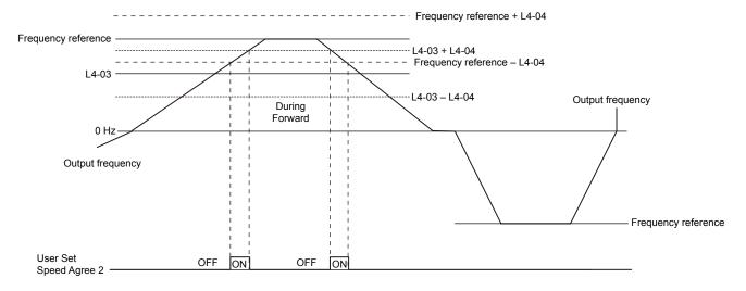
Figure i.8 User-Set Speed Agree 2 Example with a Positive L3-04 Value
