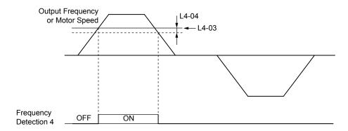
Figure i.10 Frequency Detection 4 Example with Positive L3-04 Value
