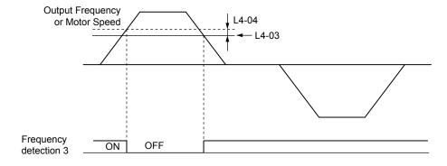
Figure i.9 Frequency Detection 3 Example with a Positive L3-04 Value
