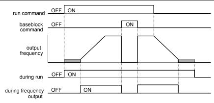
Figure i.12 During Frequency Output Time Chart
