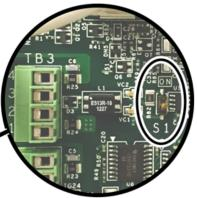
BACnet 120 ohm termination DIP switch S1. Located on Bypass Control Board A2.
