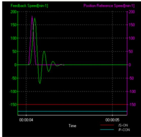
Figure 7: Untuned system (Purple plot: Reference velocity, Green plot: feedback velocity)
