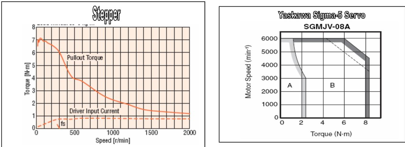
Figure 2: Comparison of torque speed curves between a stepper and a servo of comparable size.
