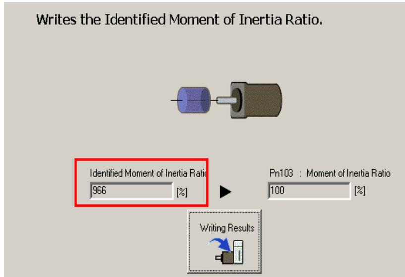
Figure 4: Inertia estimation results
