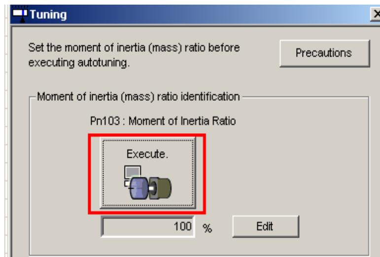
Figure 3: Inertia estimation
