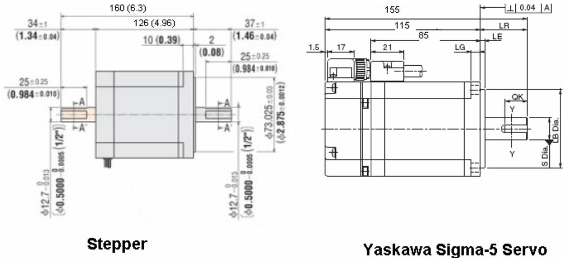
Figure 1: Comparison of motor dimensions between a stepper and a servo of comparable size.
