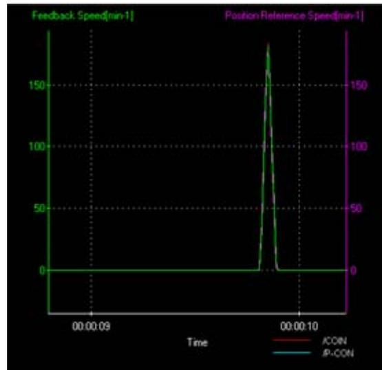
Figure 9: Autotuned system response (Purple plot: Reference velocity, Green plot: feedback velocity)
