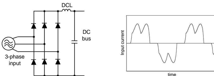
Figure 1. A 6-pulse rectifier power circuit and an input current waveform
