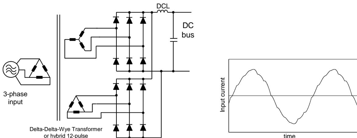
Figure 2. A 12-pulse rectifier power circuit and an input current waveform
