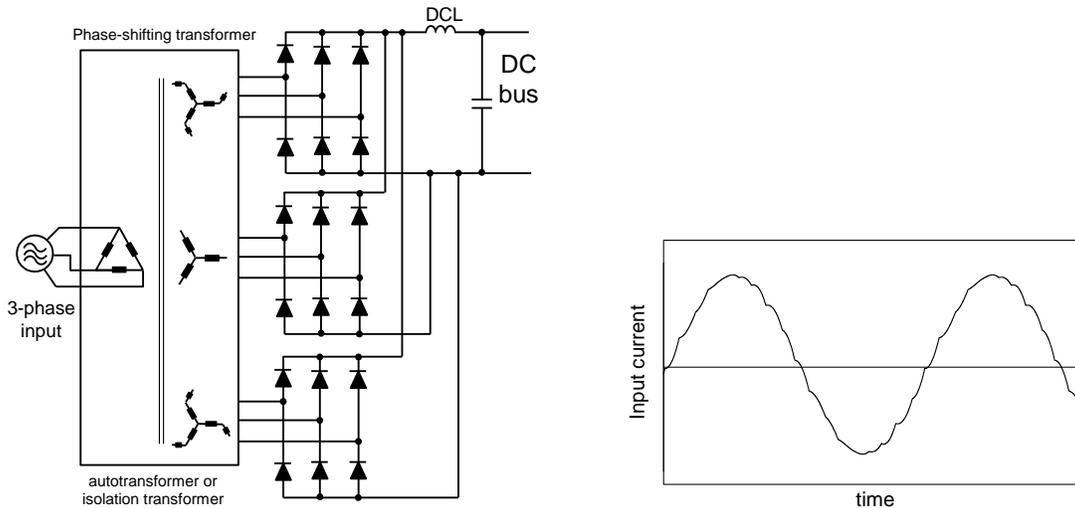
Figure 3. A 18-pulse rectifier power circuit and an input current waveform
