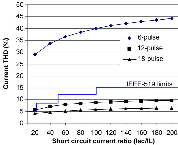
Figure 5. Input current THD according to the rectifier types, the short circuit current ratio, and a 3% DC link choke.
