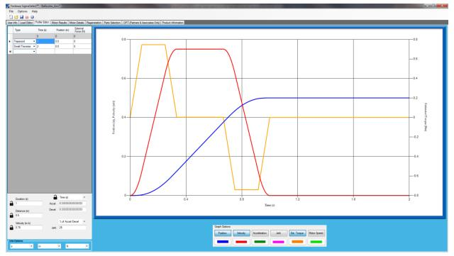
Figure 2: Speed/Torque curve from Yaskawa SigmaSelect servo sizing software plotting position (m) and velocity (m/s) on the vertical axis and time in seconds, horizontally.
